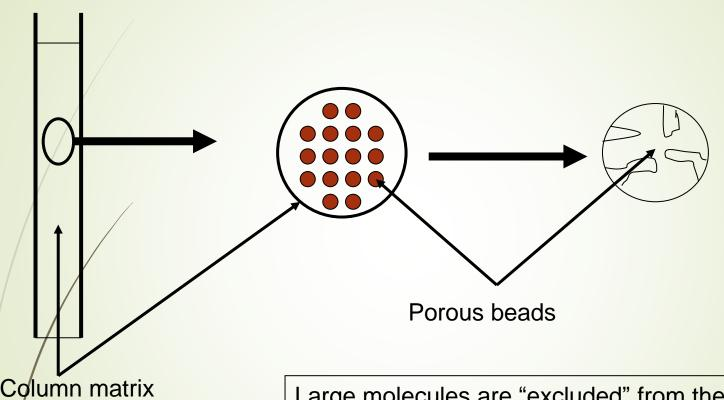
Large molecules are "excluded" from the pores and travel through the column fastest
