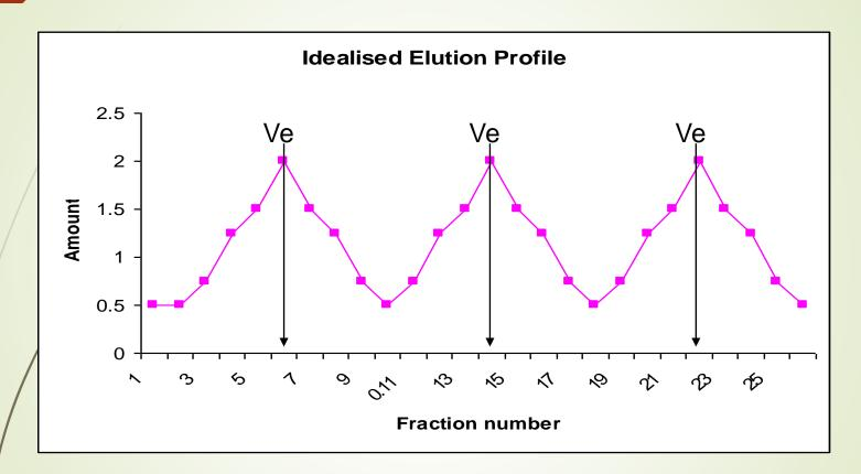
Ve = Elution volume (volume of solvent between injection and elution). Dictated by proportion of porous matrix available to molecules (Kd).
